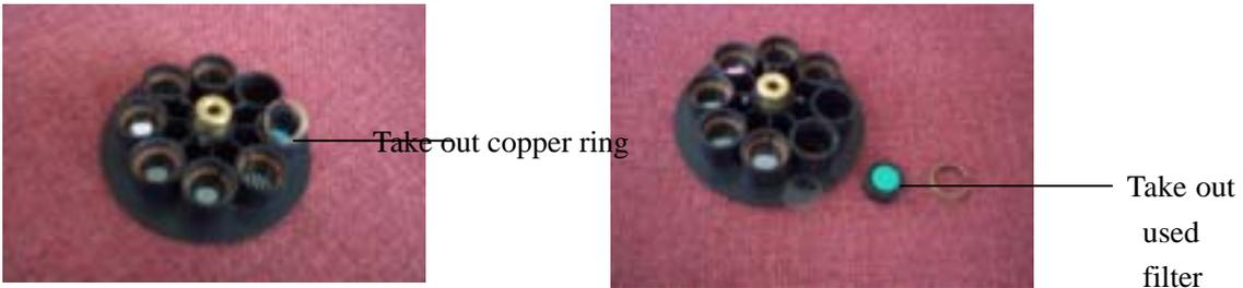
9、 Replace new filter with related wavelength, fix it with cooper ring. And the replacement is completed.
