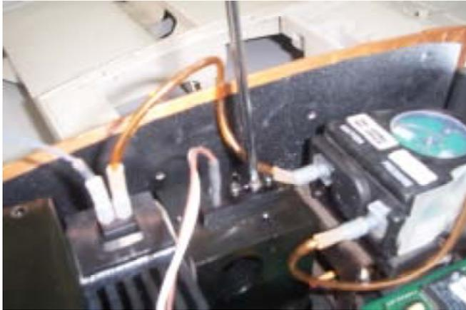
7. Fasten bolt , and place the cover of the lamp.
